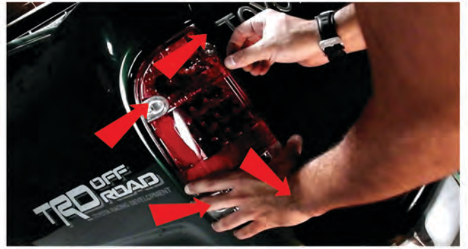
6) Seat the SPYDER headlight and reinstall the four phillips screws that secure it to the body.
