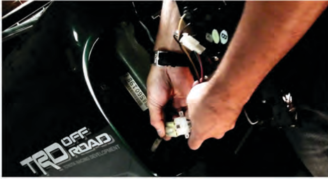
5) Connect the SPYDER tail light's wiring harness to the OEM tail light wiring harness.
