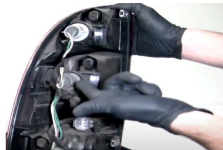
4. Remove bulb sockets and wiring harness.
