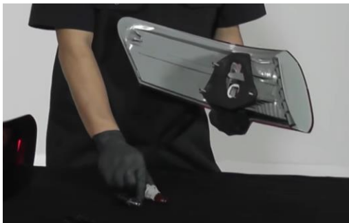
21. Remove brake and turn signal socket from OEM tail light.
