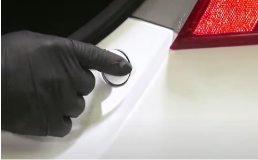
34. Reinstall fascia (1x) 10mm bolt and cap.
