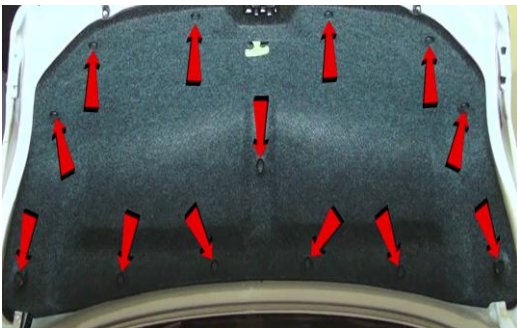
33. Reinstall (13x) plastic retainers.
