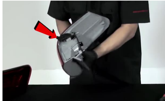
20. Remove fascia clip from OEM tail light.
