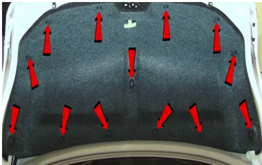
13. Remove (13x) plastic retainers.
