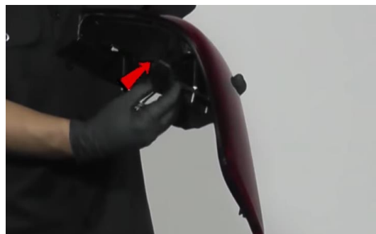
22. Install fascia clip onto Spyder tail light.
