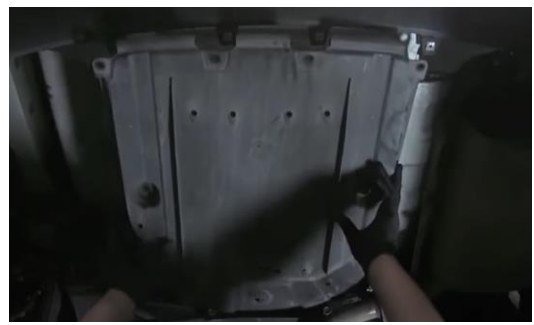
37. Reinstall underbody panel and reinstall (7x) 10mm bolts and (2x) 12mm nuts.
