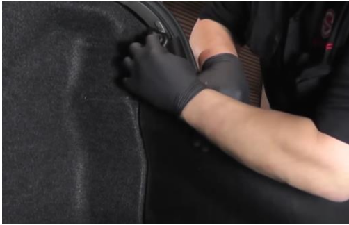
31. Reinstall trunk panel and grocery hook (1x) 8mm bolt.
