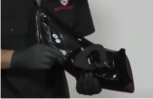
23. Install turn signal into Spyder tail light.
