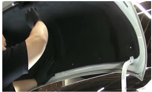
32. Reinstall decklid liner.
