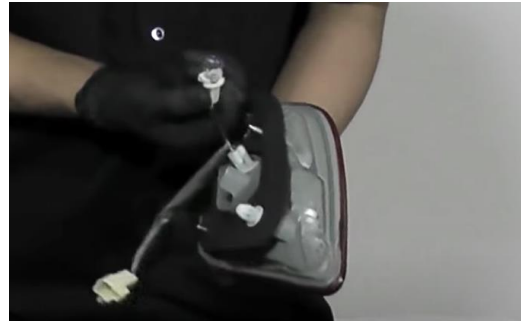
18. Remove reverse bulb from OEM tail light. (Never touch bulbs with bare hands)
