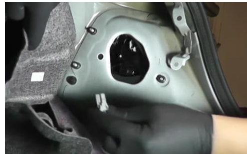
4. Disconnect tail light harness.
