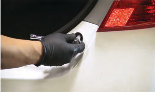
41) Reinstall [1x] 10mm bolt to secure the fascia on either side of the trunk opening.
