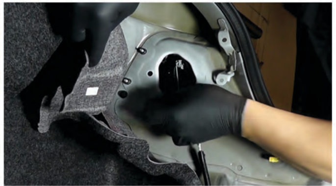
32) Reconnect the outer tail light harness.
