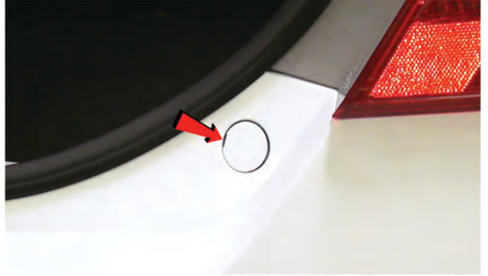
6) Remove [1x] plastic fascia cap on each side of the trunk opening.
