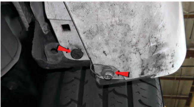
9) Remove [2x] 10mm bolts securing the bottom corner of the rear fascia on each side.
