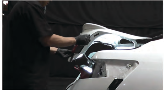
20) Unseat and remove the inner tail light.
