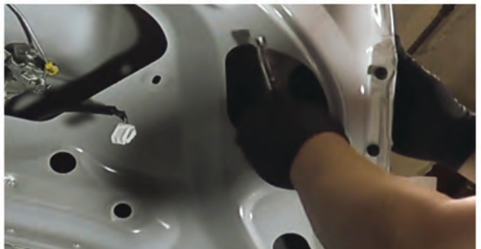
34) Reinstall [3x] 10mm nuts to secure the inner tail light.
