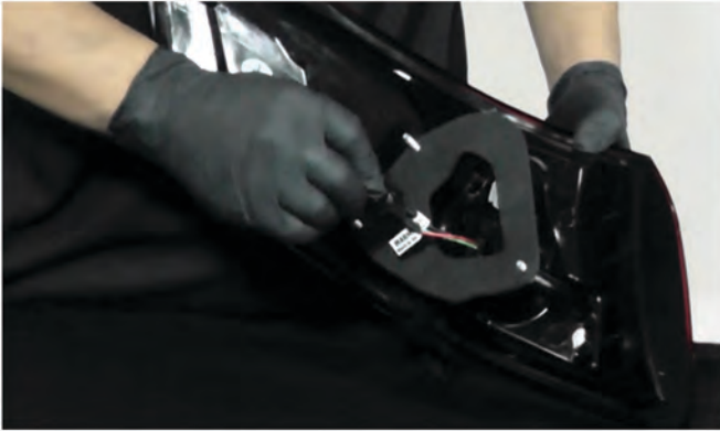
29) Install the socket insert into the brake lamp socket. Connect the black wire side of the socket with the black wire side of the insert to ensure correct polarity.
