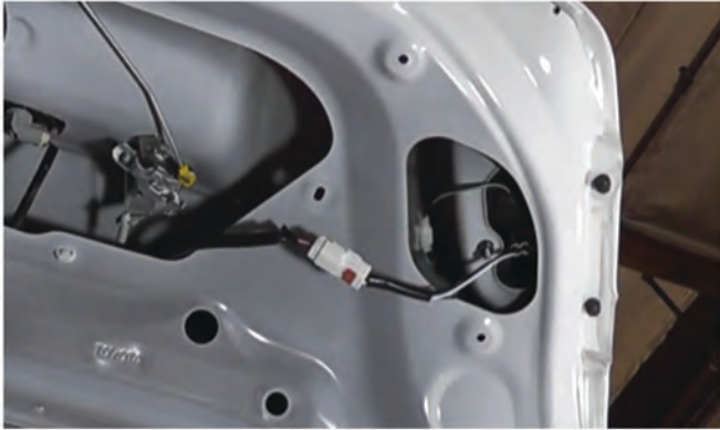
35) Reconnect the inner tail light harness.
