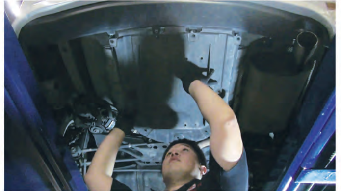
12) Remove the underbody tray and set it aside.
