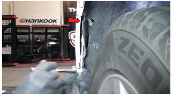
8) Remove [1x] 10mm bolt securing the fascia accessible through the hole in the rear fender liner on each side.
