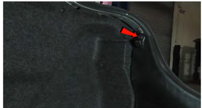
2) Remove [2x] 8mm bolts recessed in the grocery hook securing the trunk liner panel.
