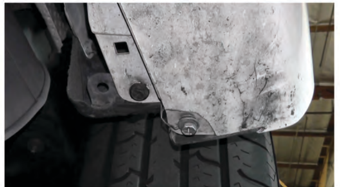
44) Reinstall [2x] 10mm bolts at the bottom corner of the fascia on each side.
