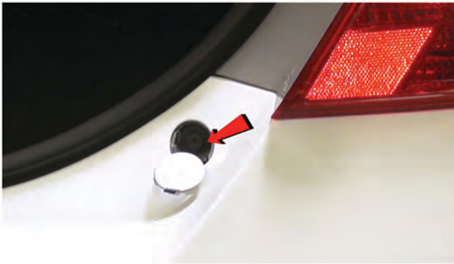
7) Remove [1x] 10mm bolt under the cap.
