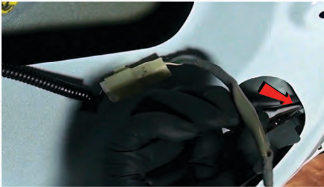
19) Use needle-nose pliers to release the final retainer tab securing the inner tail light.
