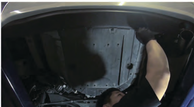
45) Replace the underbody panel. Reinstall [4x] 10mm bolts, [3x] 10mm nuts and [2x] 12mm nuts to secure the underbody panel and the fascia.
