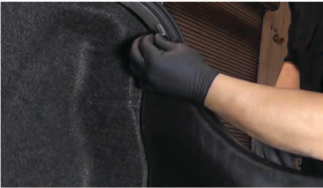
37) Reinstall [1x] 8mm bolt recessed in the grocery hook on each side to secure the trunk liner panel.
