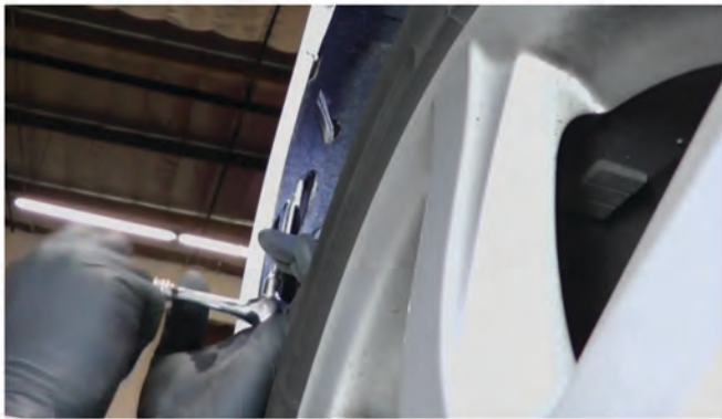
43) Reinstall [1x] 10mm bolt accessible through the hole in the rear fender liner to secure the fascia.
