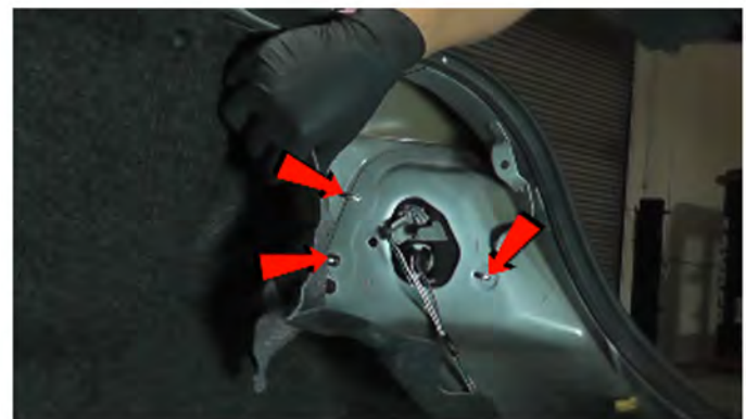
4) Remove [3x] 10mm nuts securing the outer tail light.
