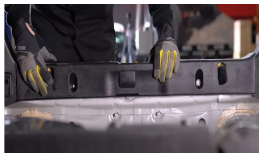
34. Reinstall rear trunk panel and (2x) plastic clips.
