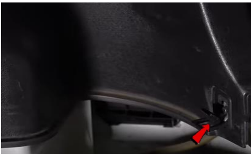
33. Reinstall (1x) 10mm bolt and plastic cover.
