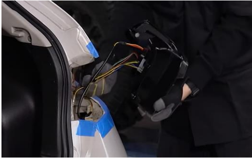
13. Tuck in remaining wires. (Note there will be (2x) unused wires for US models)
