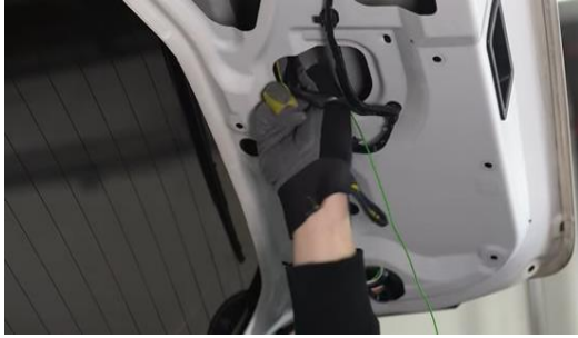
29. Push in wires and route remaining green wire to license plate light.
