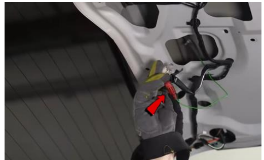
30. Tap green wire to factory black wire with white stripe. Reinstall License plate socket.
