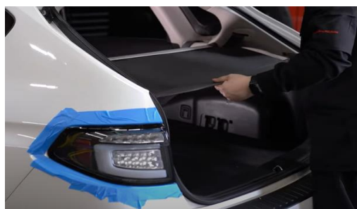
37. Reinstall security shade.
