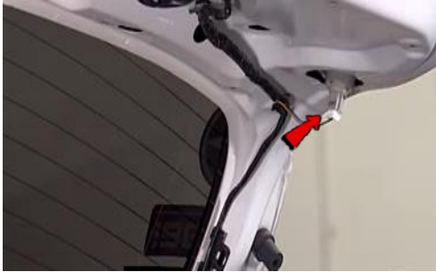
23. Remove inner tail light socket.
