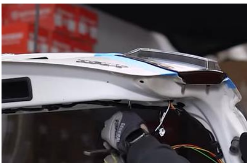
27. Reinstall (3x) 8mm nuts securing inner tail light.
