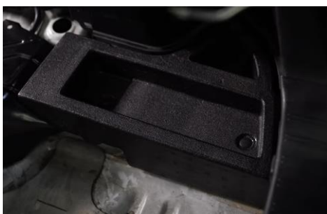
34. Reinstall spare tire foams and (2x) retaining clips.
