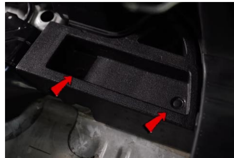
2. Remove (2x) retaining clips securing spare tire foams.
