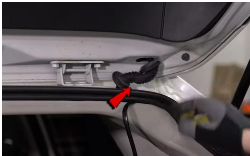
19. Loosen top and bottom of rubber boot.
