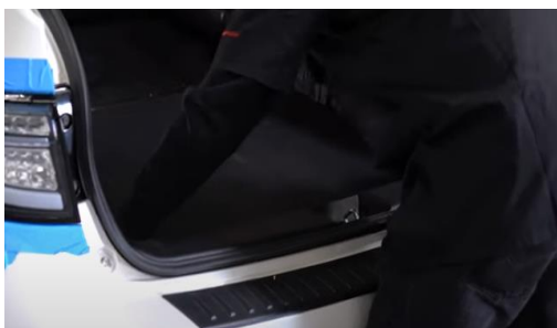
36. Reinstall trunk liner.
