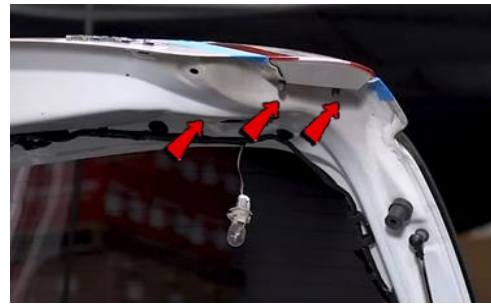
24. Remove (3x) 8mm nuts securing inner tail light.
