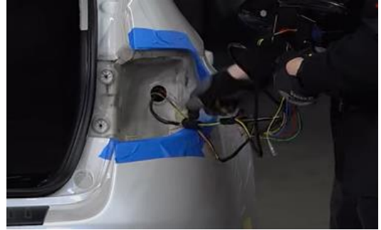
12. Push in Spyder wires and seat new rubber grommet.
