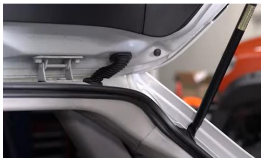
21. Push wire up and reinstall rubber boot.
