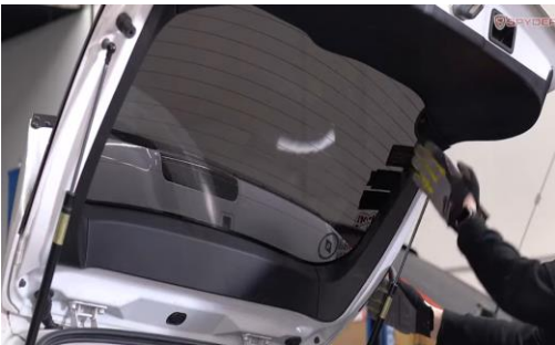
31. Reinstall (4x) hatch plastic trims.
