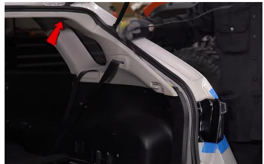
18. Route harness up through loosened panels.
