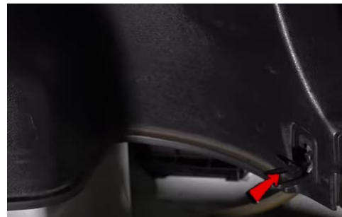
4. Remove cover to reveal bolt securing side panel.
