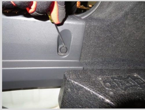
10. Peel back trunk liner to access taillight mounting hardware
