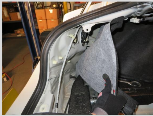
10. Peel back trunk liner to access taillight mounting hardware
