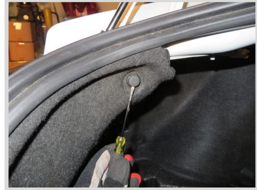
9. Remove plastic clip holding upper edge of trunk liner
