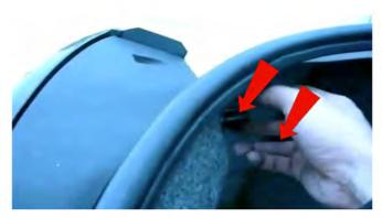
2) Locate two Black Thumbscrews behind the tail lights, securing the carpet on the inside of the trunk. Remove these thumbscrews.
