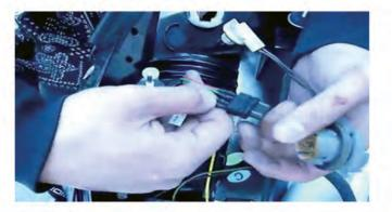
5) Locate the SPYDER tail light. Install the reverse lamp and turn signal sockets. Remove the bulb from the brake lamp socket. Connect the SPYDER wedge harness socket insert to the brake lamp socket, black wire on the black wire side of the socket.
