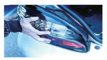
6) After reinstalling the bulb sockets and connecting the harness, seat the SPYDER tail light.
