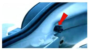
3) Peel back the trunk liner. Remove this thumbscrew behind the tail light on the inside of the trunk.
