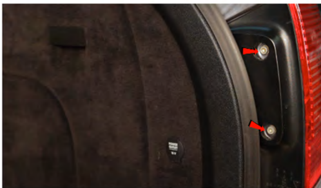
3) Remove [2x] #5 Hex Key Bolts securing the tail light.
