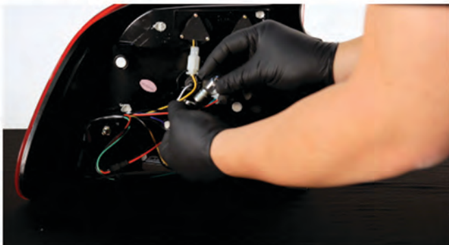
9) Transfer one bulb to the blue and black wire Spyder rear fog lamp socket.
