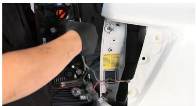
4) Remove the cargo lamp, reverse lamp, turn signal and brake lamp sockets from the OEM tail light. Never touch exposed bulbs with bare hands.
