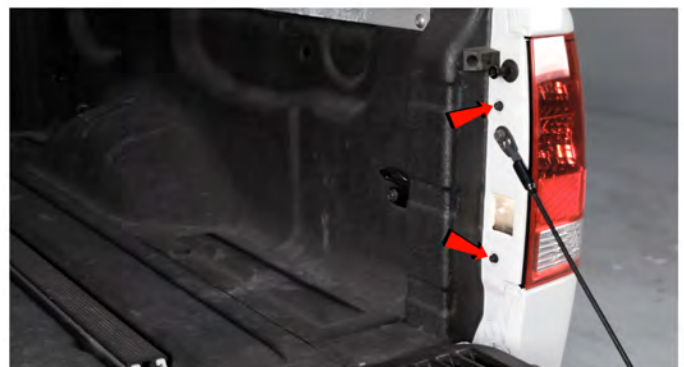
2) Remove [2x] 10mm bolts securing the tail light.
