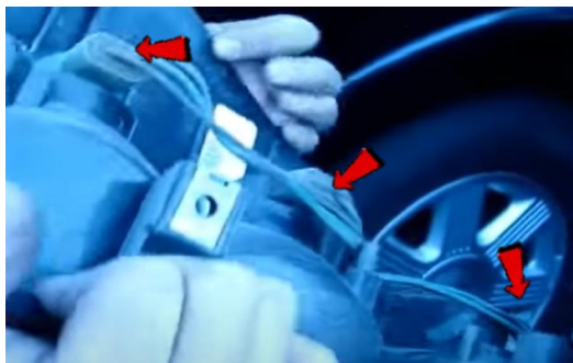
3. Remove (3x) tail light sockets.
