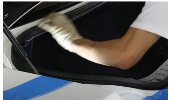
20. Reinstall weather strip.
