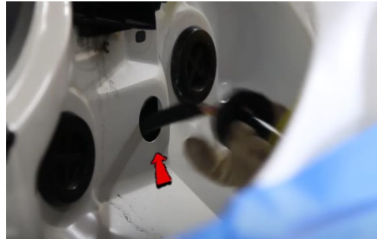
8. Unseat grommet and pull out wire harness.
