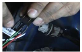
5. Connect Spyder socket insert into brake light socket. (Making sure black wire of socket is aligned to black wire of socket insert)
