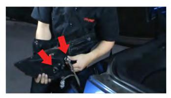
3) Next, gently push outwards from the back of the tail light to get it free. Still attached will be the tail light harness (arrows). With moderate force, twist the socket counter clockwise to unlatch it from the tail light. set OEM assembly aside.
