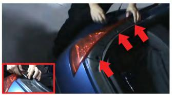
1) Start by opening your trunk and locating the (3) plastic fasteners. Using the panel popper tool or flathead, gently pry the fasteners free and set them aside for later.
