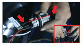
6) Next, once the brake bulb has been removed you can now insert the clip from the Spyder tail light into the brake bulb socket. Be sure you are lining up the black ground wires of both sides, installing this incorrectly can damage the harness, LED's and fuses.
