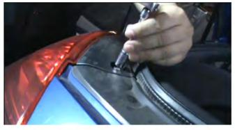
2) Once the fasteners have been removed, you will need to remove (3) 10mm nuts, shown here.
