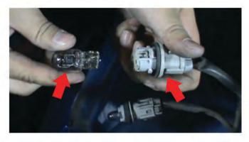
5) In order to connect the brake light function of your Spyder lights, gently pull on the brake light bulb until it pops free of the harness as shown above. Note: you can identify the brake bulb by the bulb sizing, brake bulb will be the larger bulb of the two shown.
