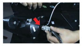
7) Now that everything is wired and connected, twist the socket from the brake harness into the tail light housing clockwise. Be sure it is seated properly to prevent any condensation in the tail lights.
