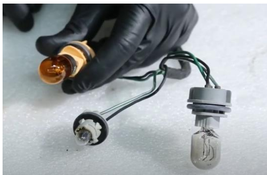
15. Replace turn signal bulb with provided amber bulb. (Never touch bulb with bare hands)
