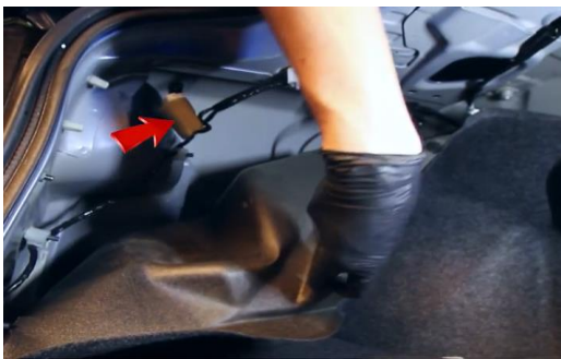
3. Pull back trunk liner to access outer tail light harness.
