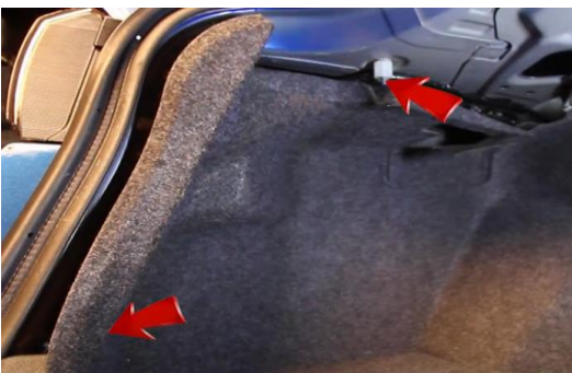
21. Reinstall trunk liner and (2x) plastic retaining screws.
