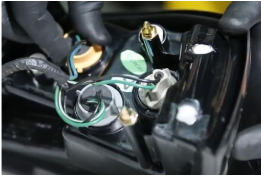
17. Seat brake, signal and side marker sockets into Spyder tail light.
