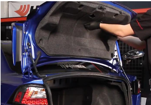
25. Align and seat trunk lid liner.
