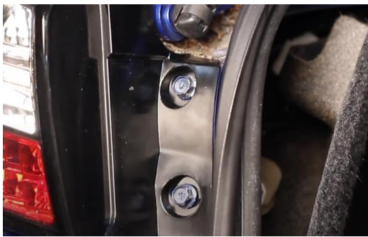
19. Reinstall (2x) 10mm bolts.
