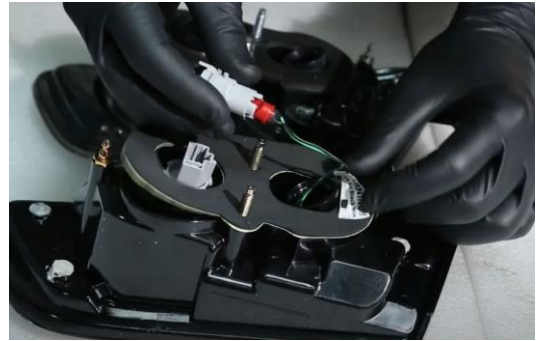
12. Unseat tail light socket and remove bulb. Transfer socket to Spyder tail light and install socket insert.
