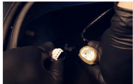
4. Disconnect outer tail light harness.
