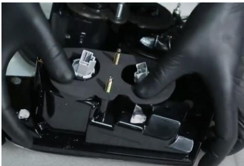
13. Peel backing from weather seal and stick to Spyder trail light.
