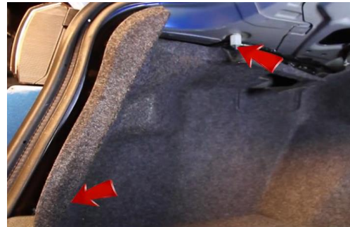
2. Remove (2x) plastic retainers.
