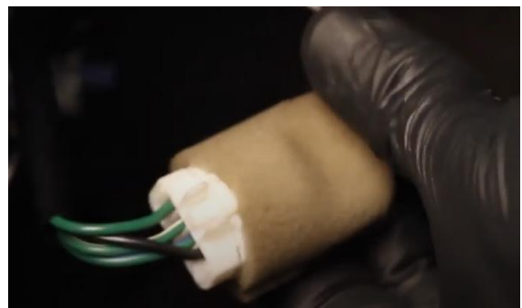
20. Connect outer tail light harness.
