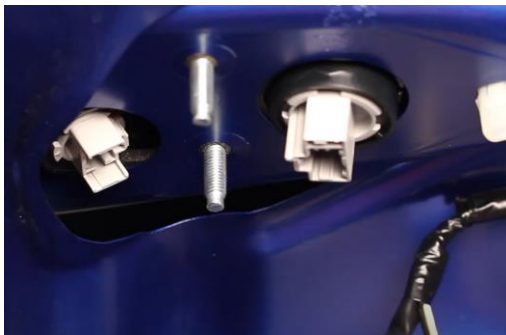
9. Disconnect inner tail light harness.
