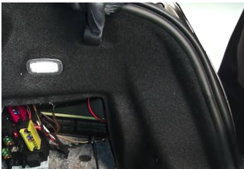
13. Seat trunk liner and install grocery hook.
