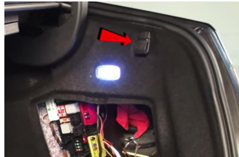
2. Remove grocery hook using panel popper.
