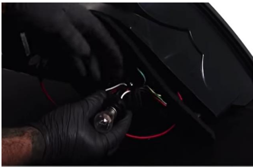
9. Install reverse bulb into Spyder reverse socket and reinstall socket.
