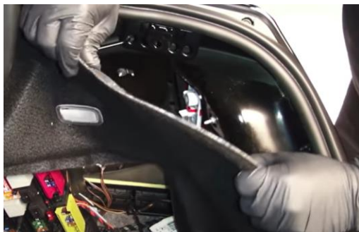
3. Pull back trunk liner to access tail light.
