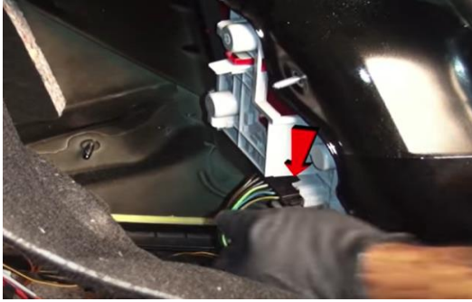
5. Disconnect wiring harness.
