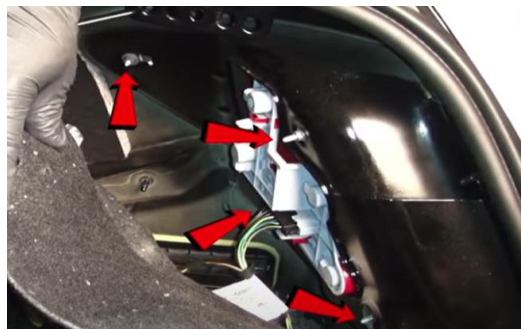
4. Remove (4x) 8mm nuts securing tail light.
