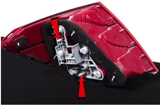
7. Squeeze tabs to release bulb plate from oem tail light.
