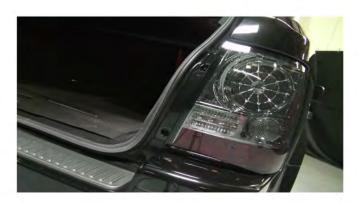
4) Reseat the tail light assembly by pressing it into place and being sure to line it up flush with the body. Reinstall the two screws and you're done!
