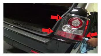
1) Open your trunk to reveal the tail light assembly. Using a flat head screwdriver, remove the two screws holding the light in place (arrow 1). Once removed, you will need to pry the assembly free. If removal by hand proves difficult, you may also use the flat driver with a towel or cloth around it to gently and carefully pry the assembly free (arrow 2).
