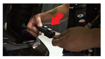
3) With the new light in hand, attach the Spyder harness to the OEM harness, The connector should \*click\* in place.
