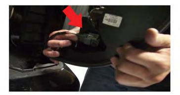
2) Once you have unseated the tail light, flip the light over. Attached will be the OEM harness. There is usually a small pressure clip/latch attched to the harness that needs to be squeezed together in order to release the harness.Squeeze, then pull apart. Once this is done, set OEM assembly aside.
