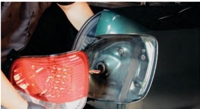
27) Seat the wiring harness grommet to properly seal the body.
