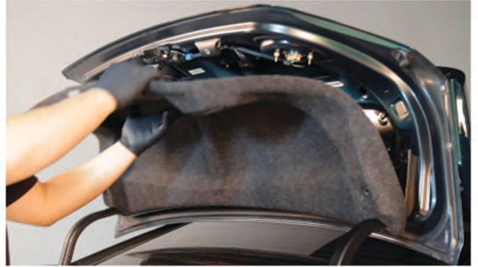
12) Unseat and remove the decklid liner.
