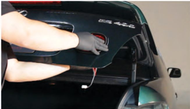
19) Seat the Spyder inner tail light, taking care not to pinch the harness.
