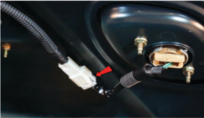
13) Disconnect the inner tail light wiring harness.
