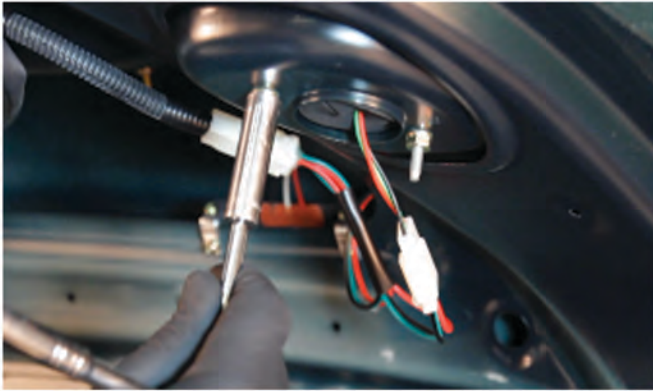
23) Reinstall [2x] 10mm nuts to secure the inner tail light.
