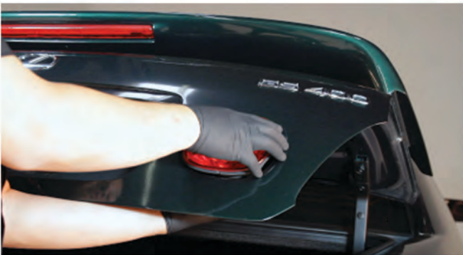
15) Unseat and remove the inner tail light.
