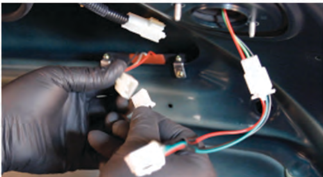
21) Reconnect the resistor pack to the Spyder inner tail light.
