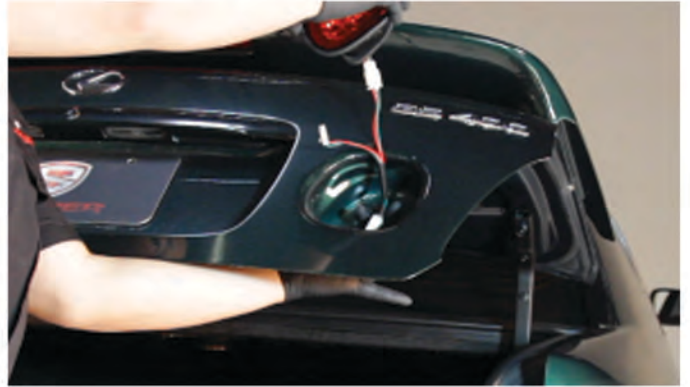
18) Feed in the Spyder inner tail light wiring harness.
