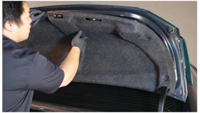
24) Seat the decklid liner panel.
