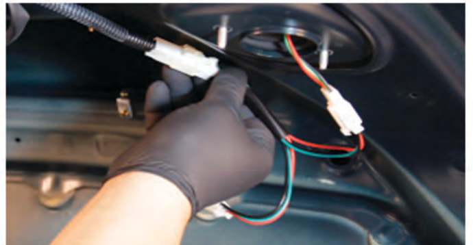
22) Connect the Spyder inner tail light to the inner tail light wiring harness.
