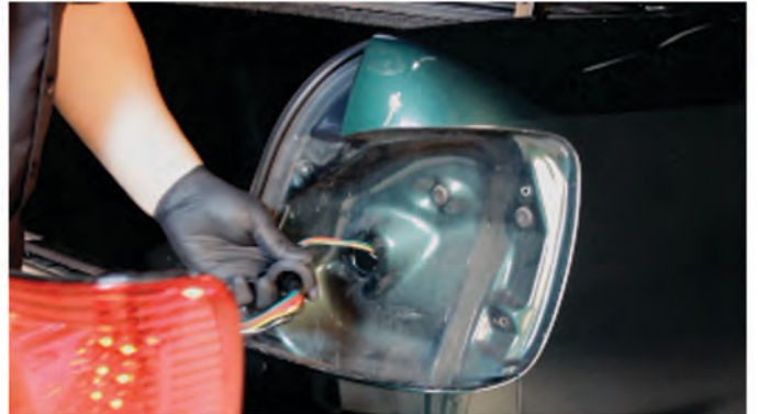
26) Feed in the Spyder outer tail light harness, being careful not to pinch it.
