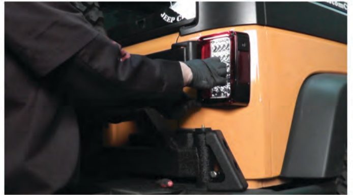
6) Reinstall [2x] Phillips Screws to mount the tail light.
