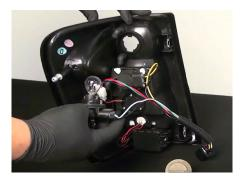
• Install reverse bulb into Spyder tail light socket with black and white wire.
