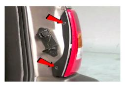
• Remove (2x) philips screws.
