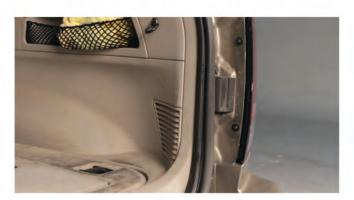
9) Reinstall the two T-20 Torx screws.
