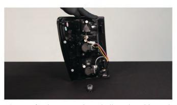
6) Transfer the reverse lamp bulb to the white and black wire reverse socket of your Spyder tail light, then reinstall the socket. Now your Spyder tail light is ready to install.
