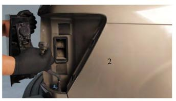
4) Disconnect the wiring harness.
