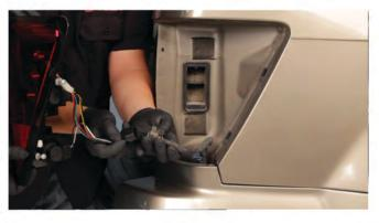
7) Connect the Spyder tail light to the OEM wiring harness.
