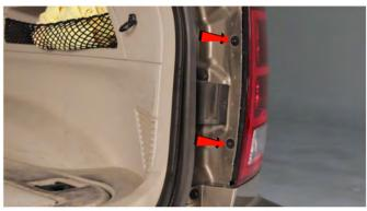
2) Remove the [2x] T-20 Torx screws securing the tail light.
