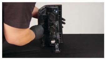
5) Remove reverse bulb socket from the OEM tail light. Remove the reverse bulb from its socket. Never touch exposed bulbs with bare hands.
