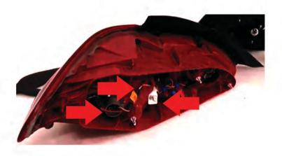
3) Once the foam seal has been removed from the tail light assembly, this will expose the bulb sockets and wire harnesses. The spyder light will re-use the light harness and bulbs. First start by pulling the white clip forward to loosen the wires. Then, twist and remove each bulb socket from the assembly. The light wires will be held in place by retaining hooks, simply slide the wires free and remove the harness.
