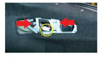
6) Carefully mount the new Spyder LED tail light back onto the body of your car. Make sure to line up the holes and replace the 4 10mm screws. Reconnect the new harness to the OEM harness as well. Lastly, replace the tail light panel cover, test for connectivity, and you're done. You have now successfully installed your new LED tailights to your Hyundai Genesis coupe.
