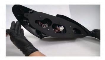
5) Make sure that the harness/bulbs are secured, pushed into the holes and locked into place. Now that the wires/bulbs are in place and the bulbs have been placed in the correct sockets, replace the black gasket that was removed from the Spyder LED tail light assembly. Match the holes up and make sure it is secured onto the mounting bolts.
