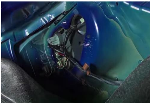
9. Disconnect tail light harnesses and remove turn signal and brake light socket.
