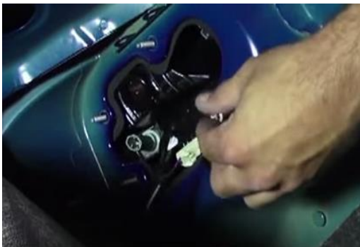
13. Reinstall (4x) 10mm nuts securing tail light.
