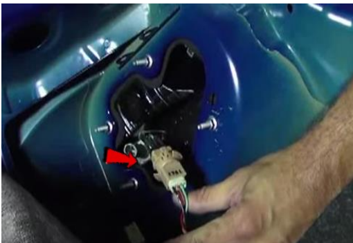
15. Install Spyder brake socket insert into brake socket. (Making sure to align black wire of socket insert to black wire of socket)
