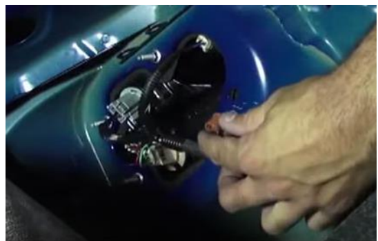
16. Install turn signal and brake sockets into Spyder tail light. Install (2x) harness plugs into Spyder tail light.
