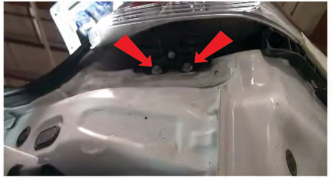
12) Remove the two 10mm bolts securing the tail light bracket.
