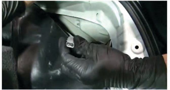
18) Remove the brake lamp bulb from the brake lamp socket. Connect the empty socket to the brake lamp wiring harness.
