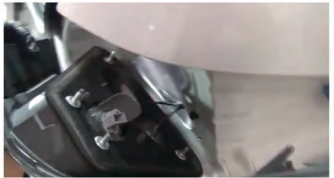
14) Disconnect the turn signal and reverse lamp wiring harnesses from the OEM tail light, then remove the tail light completely.
