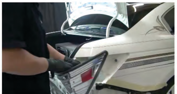
16) Reconnect the turn signal and reverse lamp wiring harnesses.
