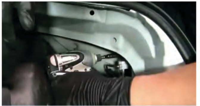
20) Reinstall the four 10mm nuts that secure the tail light to the body.
