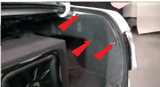
21) Replace the trunk liner and reinstall the three plastic retainers securing it.
