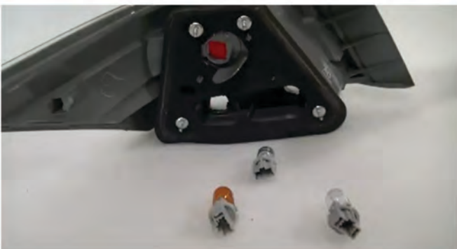
15) Remove the brake lamp socket, turn signal socket and reverse lamp socket from the OEM tail light housing. Install the turn signal and reverse lamp bulb sockets into your new SPYDER tail light.
