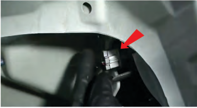
11) Disconnect the brake lamp harness.
