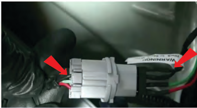
19) Insert the SPYDER tail light's brake lamp socket insert harness into the brake lamp bulb socket, being sure to align the black wire on both sides of the harness connection. Failure to line up the black wires will blow fuses and void your warranty. Insert the bulb socket and twist it into place.
