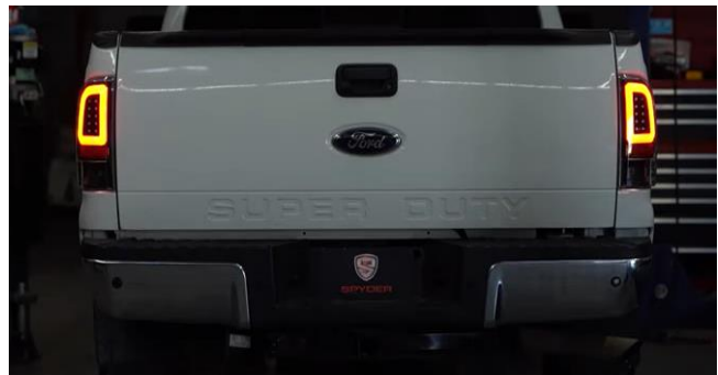
8. Turn on lights and confirm all functions are working properly. You have successfully completed the install of your new Spyder LED tail lights.
