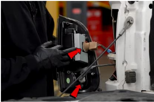
5. Install brake and reverse sockets onto Spyder tail light
