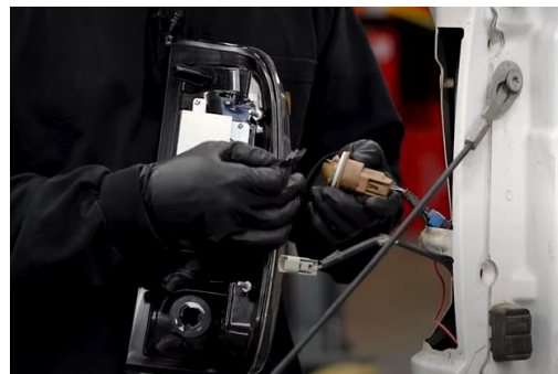
4. Remove brake light bulb from sock and install brake socket insert into brake socket. (Make sure to align black wire of socket to black wire of socket insert)
