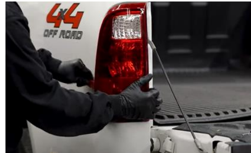
2. Unseat tail light using panel popper.
