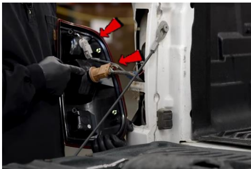
3. Remove brake and reverse light sockets. (Make sure to not touch bulb with bare hands)
