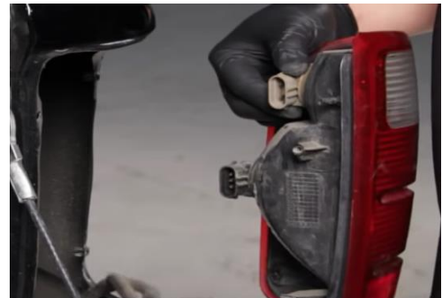
4. Disconnect Brake and reverse light harness.
