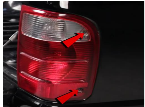
2. Remove (2x) outer phillips screws.
