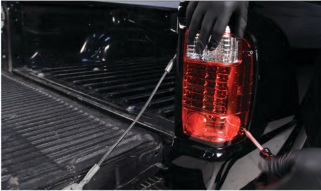
11) Reinstall [2x] outer phillips screws to secure the tail light.
