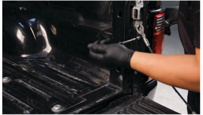
12) Reinstall [2x] phillips screws securing the tail light along the tailgate sill.
