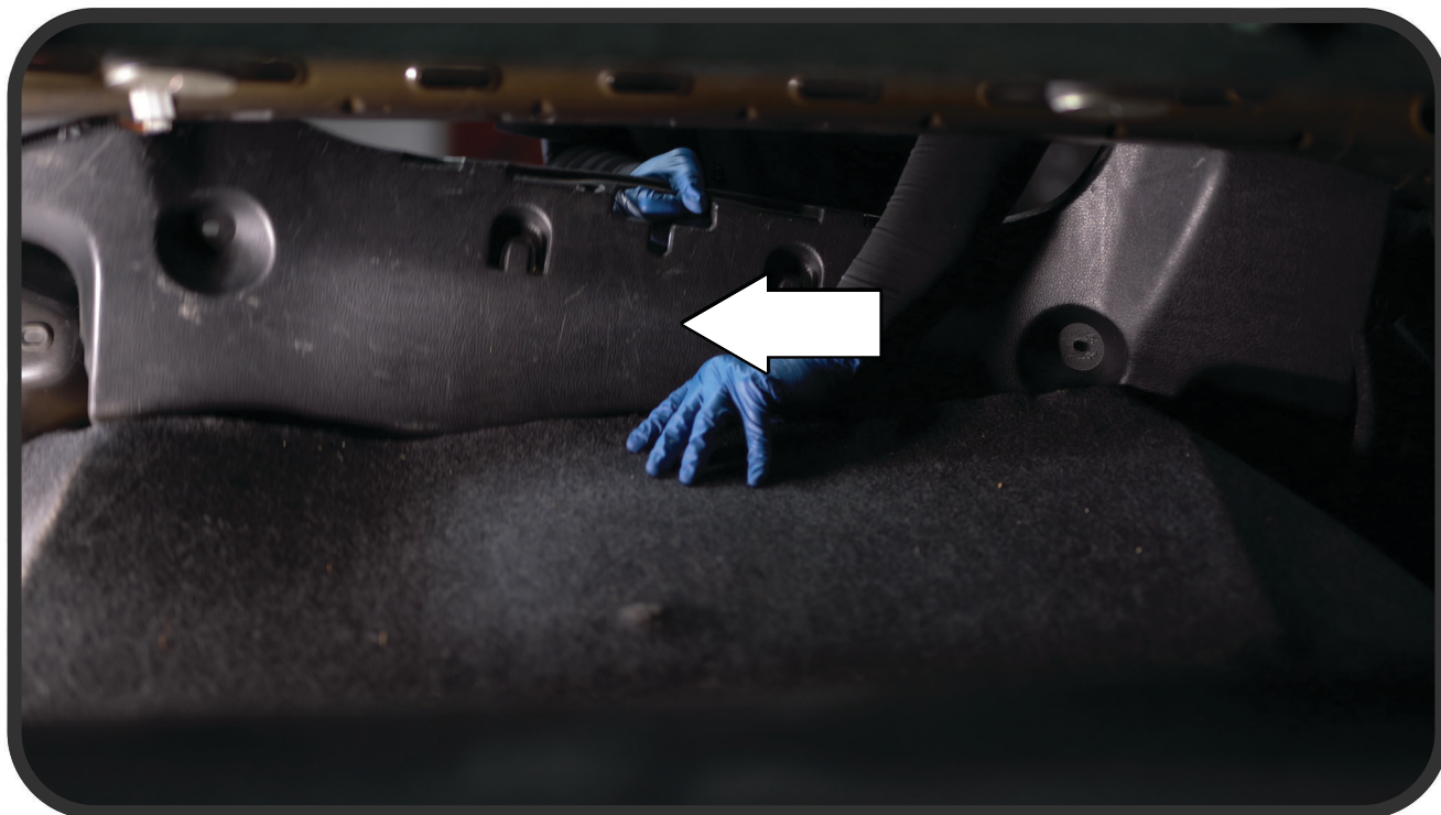
STEP 4: REMOVE THE TRUNK LINER PANEL
