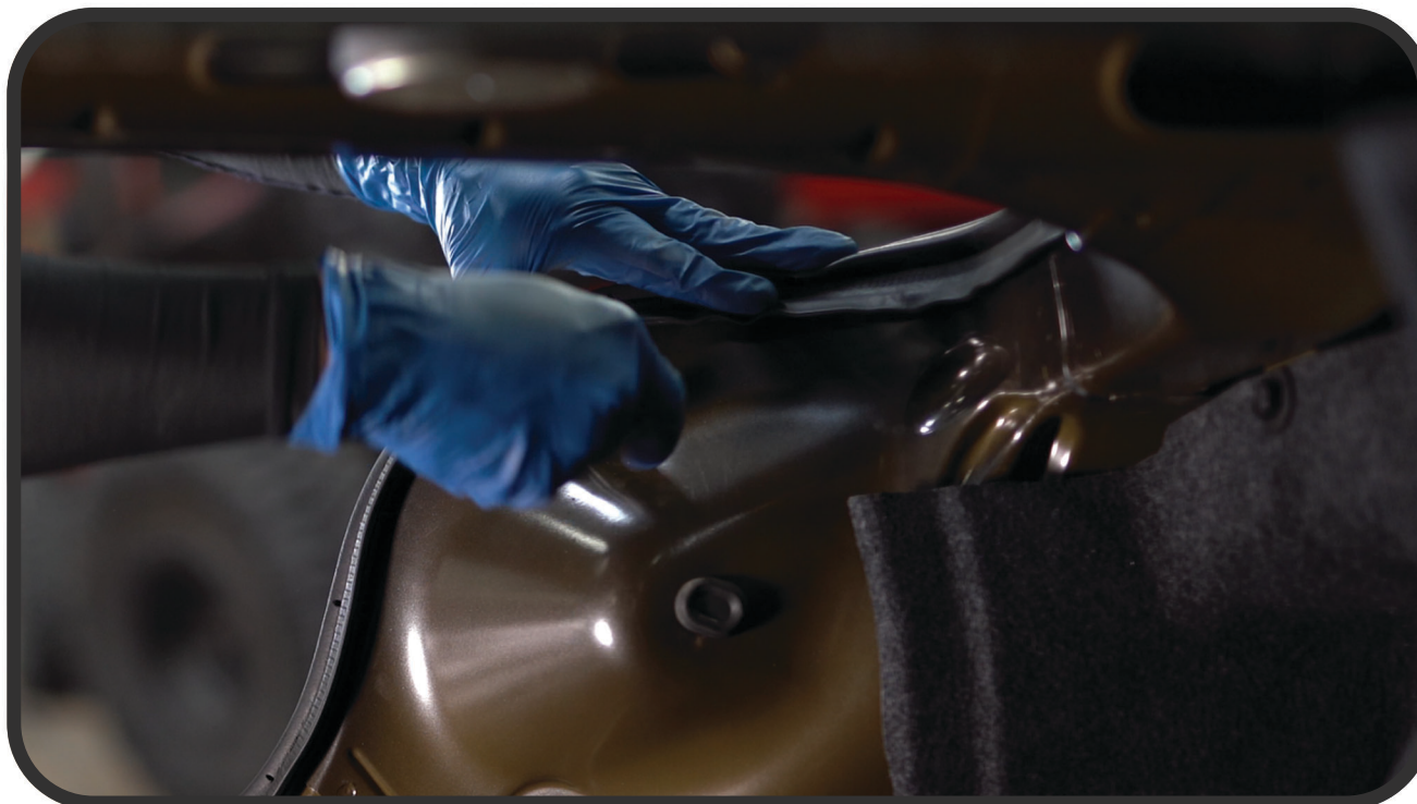
STEP 13: REINSTALL THE (3) 10MM NUTS TO SECURE THE TAIL LIGHT
