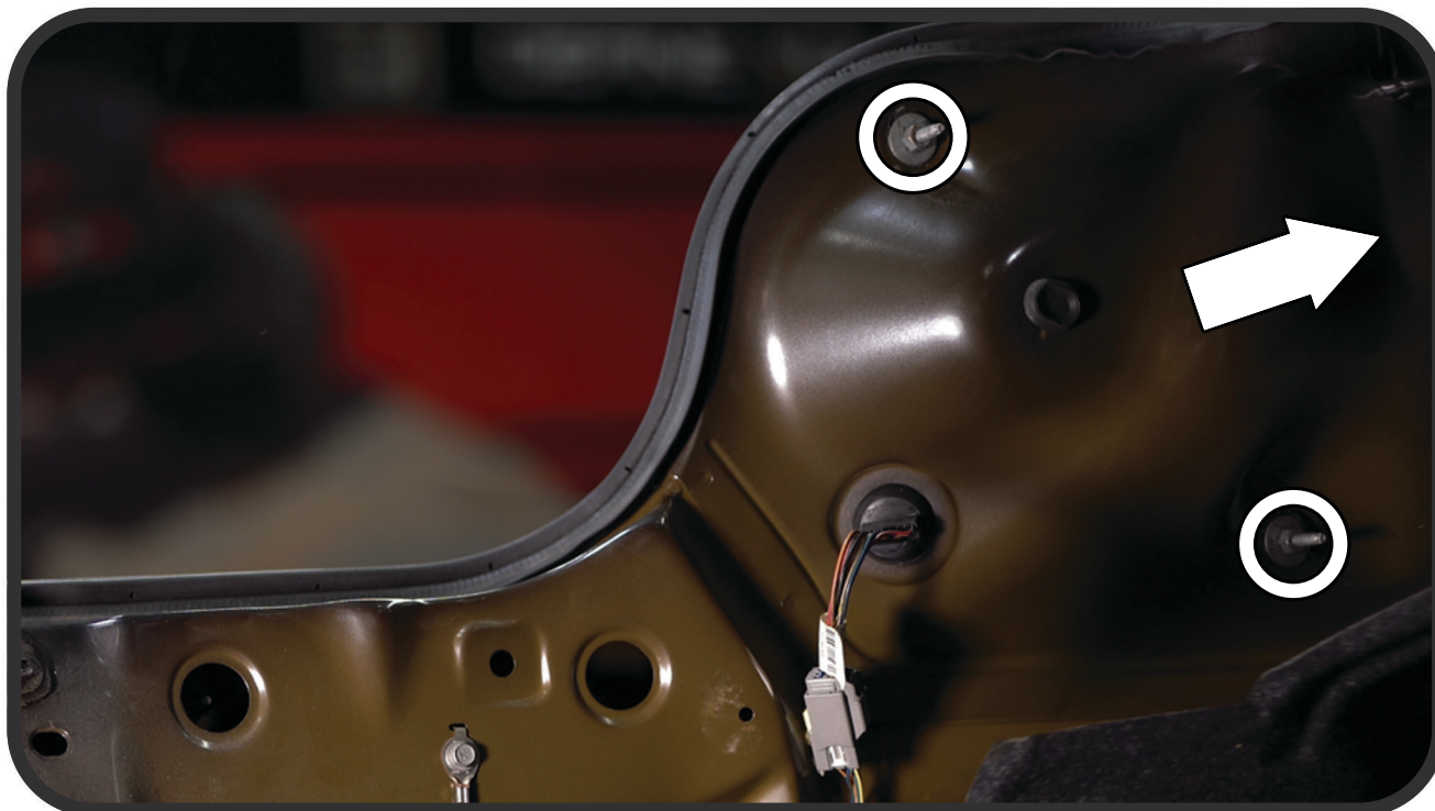
STEP 5: REMOVE THE (3) 10MM NUTS SECURING THE TAIL LIGHT
