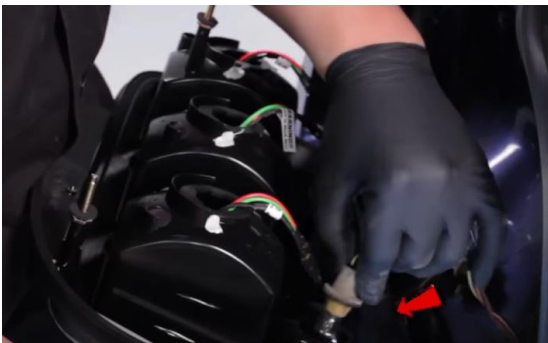
9. Install reverse light socket into Spyder tail light.
