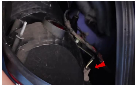
8. Remove reverse light socket.
