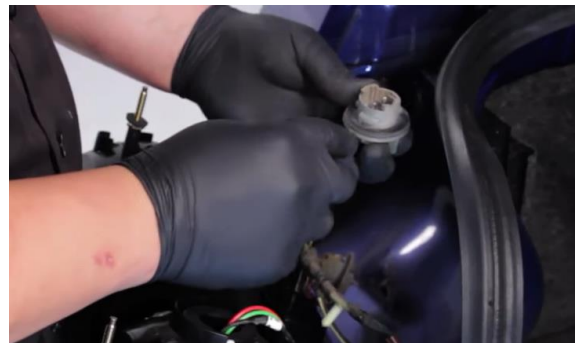
10. Remove (3x) brake light bulbs from sockets.
