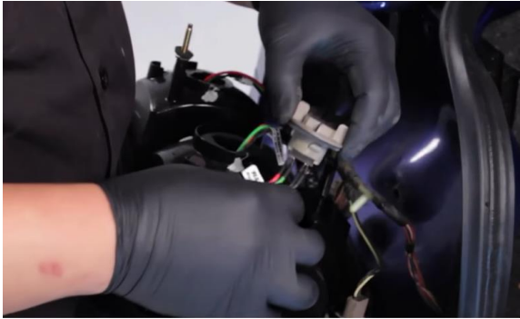
11. Install (3x) socket insert into brake bulb sockets. (Align black wire of socket with black wire of socket insert)
