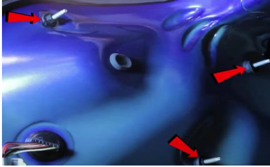
5. Remove (3x) 10mm nuts securing tail light.
