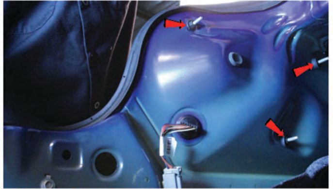
6) Remove [3x] 10mm nuts securing the tail light.
