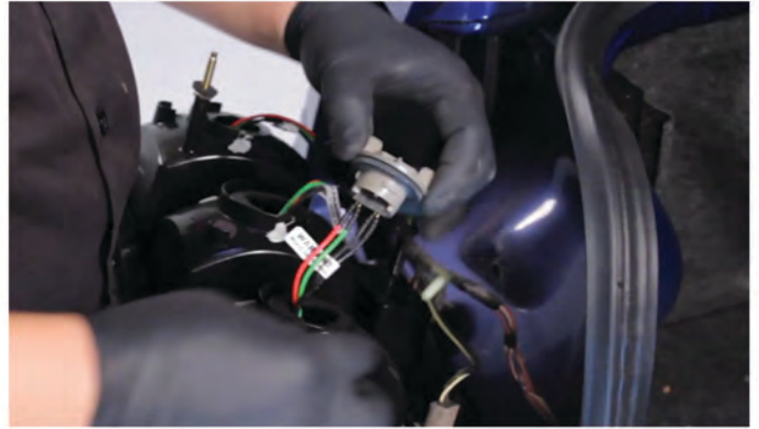
12) Install the Spyder socket inserts into the corresponding brake lamp sockets to connect the Spyder tail light. Align the black wire side of the socket insert with the black wire side of the socket to ensure correct polarity.
