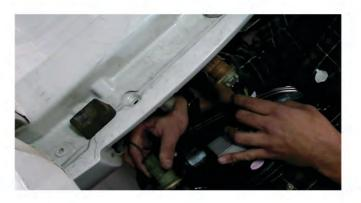
6) Install the reverse lamp socket and brake lamp socket into the Spyder tail light housing, being sure to seal the bulb sockets properly.
