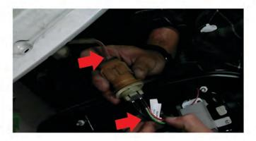
5) Locate the SPYDER headlight. Locate the wedge bulb socket insert harness. Install the wedge bulb socket insert, making sure to align the black wire side of the insert harness and the black wire side of the bulb socket harness. Failure to do so could result in electrical problems.
