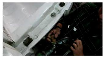
3) Remove the brake lamp and reverse lamp bulb sockets from the housing, then remove the OEM tail light housing and set it aside.
