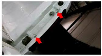
1) Open the tailgate. Remove [2x] 10mm bolts securing the tail light to the body.
