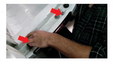
8) Reinstall [2x] 10mm bolts securing tail light, then close the tail gate.
