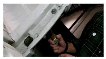
4) Remove the brake lamp bulb from the socket.
