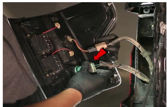
6. Plug reverse light socket into Spyder tail light.
