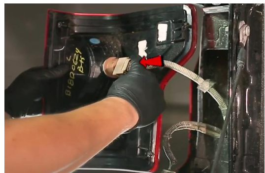
4. Unclip brake light harness.
