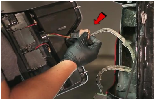
5. Connect brake light harness to Spyder tail light.
