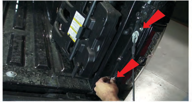
6) Reinstall the two 8mm bolts to secure the tail light.
