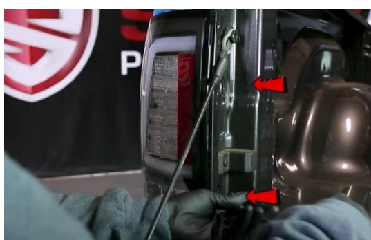
6. Reinstall (2x) T25 torx screws.
