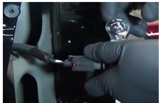
4. Remove brake bulb from socket.
