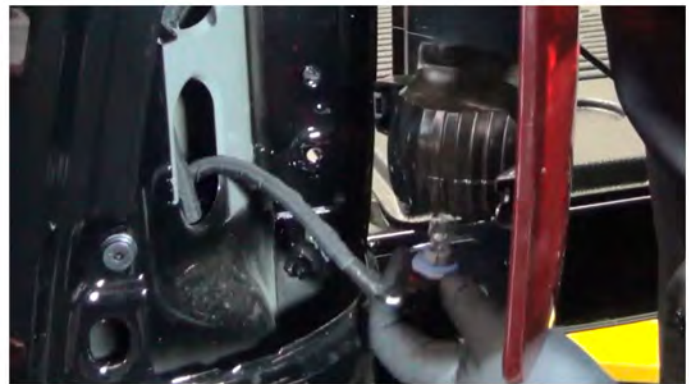
4) Remove the reverse lamp socket from the tail light. Never touch exposed bulbs with bare hands.
