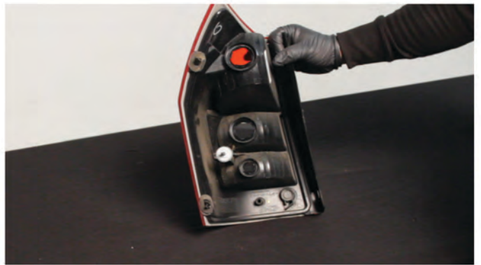
8) Remove the harness from the OEM tail light.
