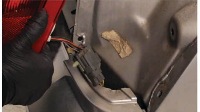
6) Disconnect the tail light wiring harness.
