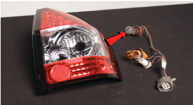
9) Remove the brake lamp bulb from its socket.
