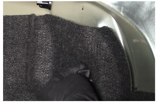
12. Reinstall (1x) thumbscrew securing trunk carpet liner.
