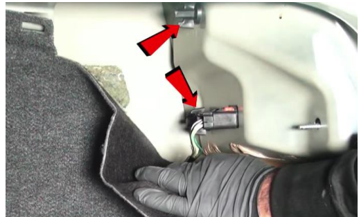
2. Pull back carpet liner and remove (2x) thumbscrews.
