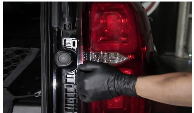
4. Unseat tail light and pull through harness.
