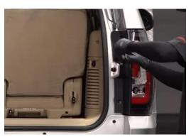
8. Reinstall (2x) phillips screws securing tail light.
