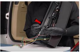
6. Install bulb in Spyder reverse tail light socket.
