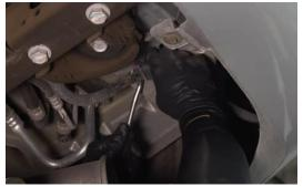
1. Under rear bumper using panel popper remove connector from body panel.
