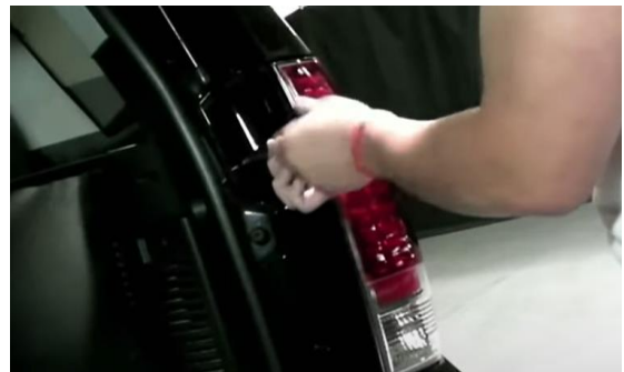
8. Reinstall (2x) phillips screws securing tail light.
