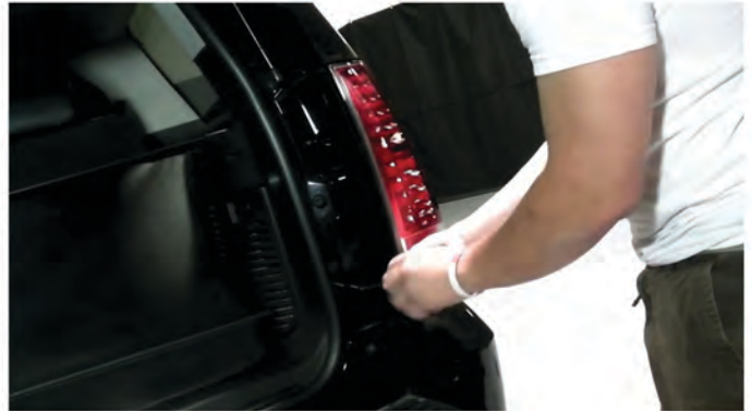
8) Reinstall [2x] phillips screws to secure the tail light.
