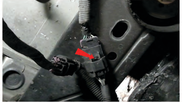
6) Connect the Spyder harness to the tail light harness in place of the bulb socket harness.
