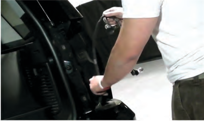
5) Remove the bulb socket harness and set it aside.
