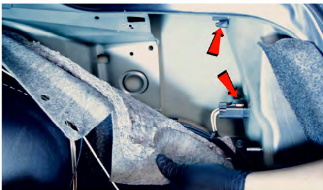
3) Remove [2x] Thumbscrews securing the tail light.
