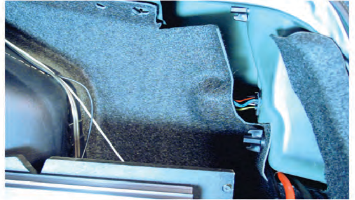
12) Replace the trunk liner and install [1x] thumb-screw.
