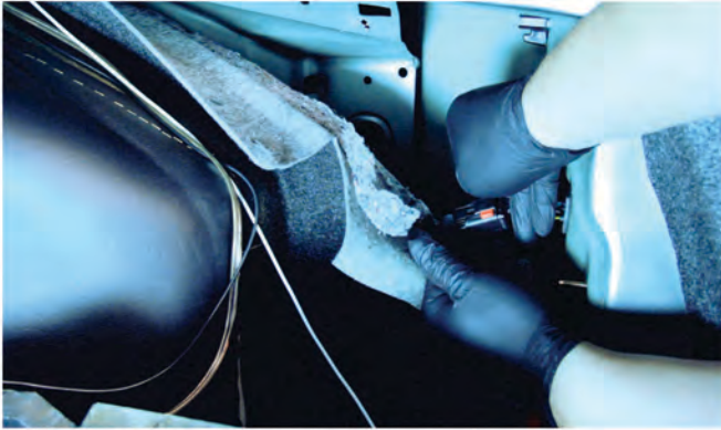
11) Reconnect the tail light wiring harness, then lock the red tab.
