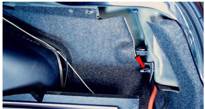
2) Remove [1x] Thumbscrew that secures the trunk liner, then peel back the liner for access.
