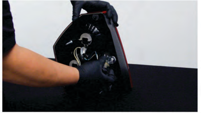
6) Remove the reverse lamp socket, then remove the bulb from the socket. Never touch exposed bulbs with bare hands.
