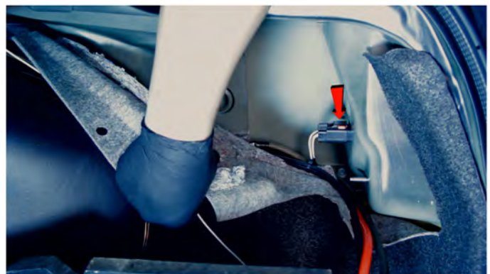
4) Unlock the red tab, then disconnect the tail light harness.
