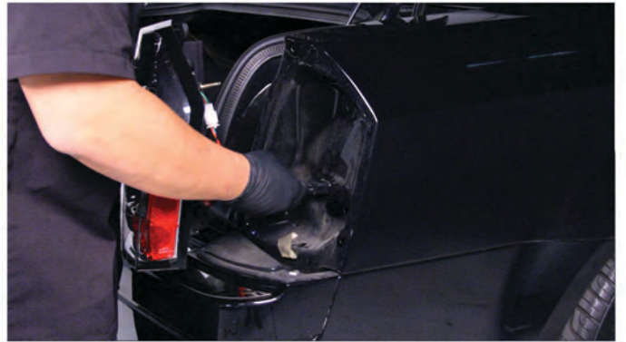
8) Feed the harness through the opening, being sure to seat the wiring harness grommet.
