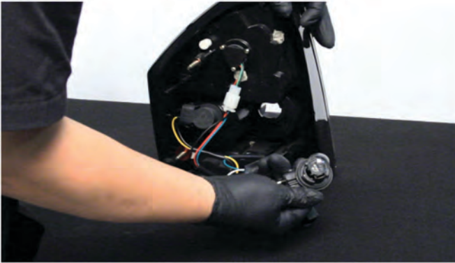
7) Transfer the reverse bulb to the black and white wire reverse socket of the Spyder tail light. Then reinstall the socket.
