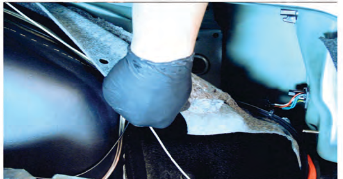
10) Reinstall [2x] thumbscrews to secure the tail light.
