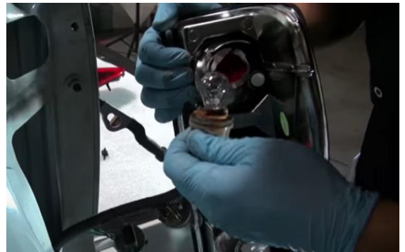
4. Install (3x) bulb sockets into Spyder tail light.
