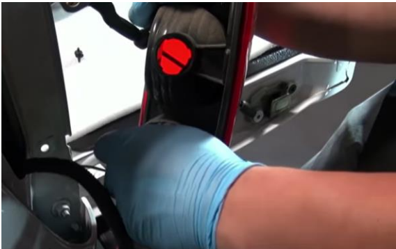
3. Remove (3x) bulb sockets from tail light. (Never touch bulbs with bare hands)
