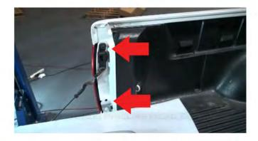
2) Located here are the two phillips bolts that will need to be removed in order to get the OEM tail light assembly separated from the body.
