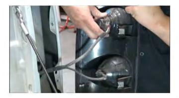
3) Once you've removed the bolt, gently pry the assmbly free. On the back of your tail light you will have 3 bulb connectors. Remove these by turning the bulb counter clockwise. Set OEM assembly aside.
