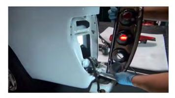
4) Pick up the new Spyder tail light, and bring it over to the bulb harness and sockets from your car. Start to replace the bulbs that used to be attached into the OEM tail light in the same order you removed them. All bulbs should placed into the same sockets they were removed from.
