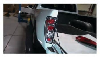
6)Reseat the tail light assembly by pressing the unit back into place. Replace the two phillips screws that were removed earlier and tighten. The tail light should be firmly in place with no movement if installed correctly. Repeat this process for the opposite side and you're done!
