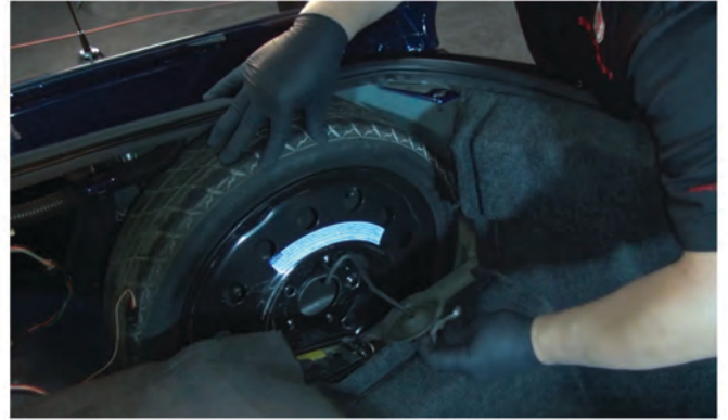
6) Remove the spare tire retainer hook, then remove the spare tire and set it aside.
