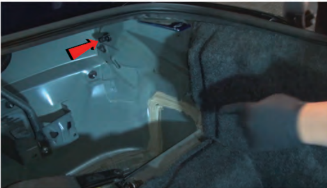
7) Remove the outer thumbscrew securing the tail light which was hidden by the spare tire.
