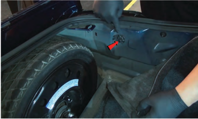
5) Peel back the trunk liner, then remove the inner thumbscrew securing the tail light.
