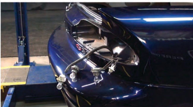
9) Remove the brake lamp, reverse lamp and turn signal sockets from the OEM tail light. Never touch exposed bulbs with bare hands.
