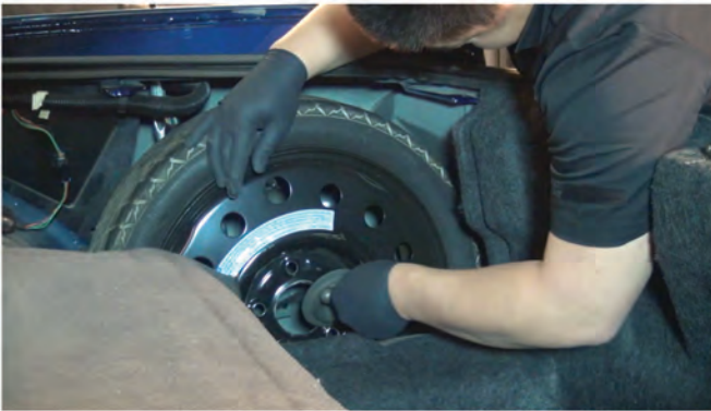
13) Reinstall the spare tire, then reinstall the spare tire retainer hook.
