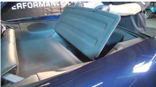
15) Seat the spare tire cover panel, then lock the three flathead retainers to secure the panel. Then reinstall the trunk separator panel.
