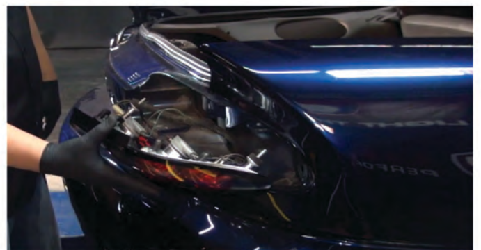
10) Install the brake lamp, reverse lamp and turn signal sockets into the Spyder tail light.
