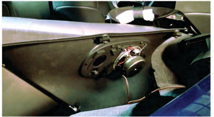
14) Reconnect the speaker harness for the spare tire cover panel.
