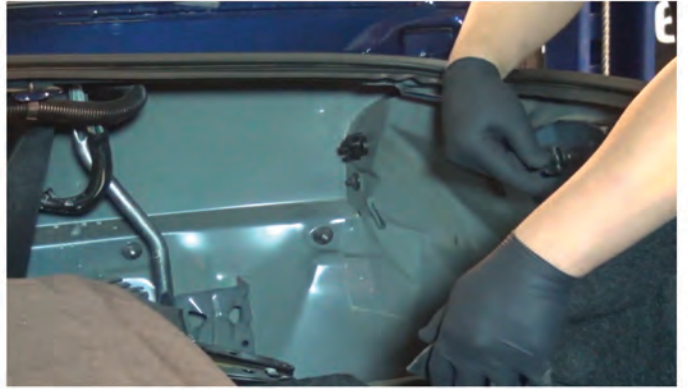
12) Reinstall [2x] thumbscrews to secure the tail light.
