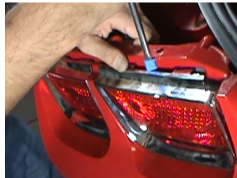
4. Release (6x) retainer tabs to remove each bezel.
