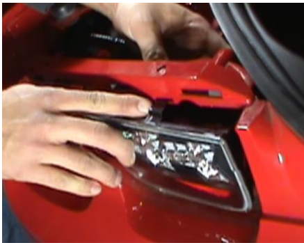
7. Seat Spyder inner and outer tail lights making sure to seat guide tabs.
