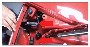
3. Gently disconnect the taillight assembly by pressing on the tabs on the harness and pulling apart. There will be a total of two per side so make sure these are disconnected before removing the light assembly.
