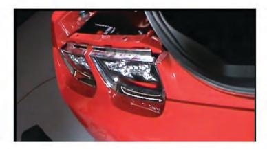
9. Replace bezels in the same order you removed them. Simply line up the mounting clips to the tail light and with even pressure press the plastic bezel back into place until you hear a click.
