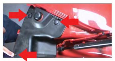
1. Using the pannel popper tool, remove the 3 plastic retainers by sliding the tool in between the covering and retainers. Pop up and remove. Set cover/retainers aside.
