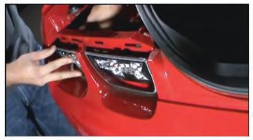
8. Once the new assembly is in place, replace all the 10mm screws and tighten down. The assembly should be a snug fit, but make sure not to over tighten the bolts and this can cause stripping and/or difficulty if you need to remove it later.
