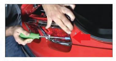
5. Continue to remove all 4 bezels from the tail light assembly keeping note the orientation and side you removed it from. Use gentle pressure (usually enough to release the clips from the body) and remove by hand.
