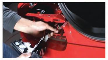
7. Slide the new Spyder tail light assembly into place of the OEM assembly. Repeat for all four sides. Always double check fitment to prevent possibly installing the left hand side on the right and vise versa.
