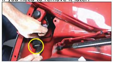
10. Once the tail lights are firmly in place, attach the new tail light harness to the OEM harness until you hear a click.
