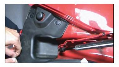
11. Replace cover panel and retainer screws. Press into place each retainer screw until it is firmly into place without movement. Repeat on both sides.
