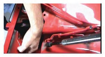
6.Once the bezels have been removed, the tail light assembly should come free. Simply push outward from the inside of the tail light assembly and remove from the body.
