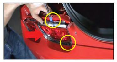
4. Locate the tabs attached to the bezel in the back of the light. Using a flat-head screw driver, gently pry out the bezel from the tail light from the top, sides, and bottom. Be careful not to break the bezel tabs.
