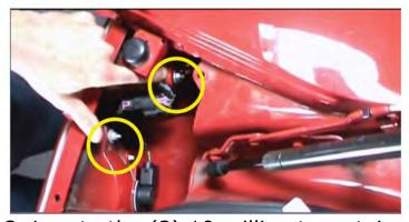
2. Locate the (3) 10 millimeter retaining nuts on each of the tailights and remove. Repeat for each light until a total of 12 10mm nuts have been removed. Set aside.
