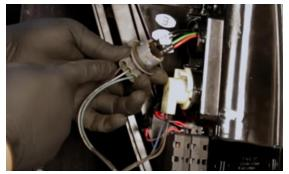
5. Install upper bulb insert into upper socket making sure again to match black wire side of insert to black wire side on socket.
