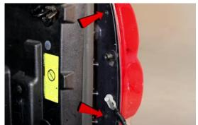
1. Remove (2x) phillips screws securing tail light to the body.
