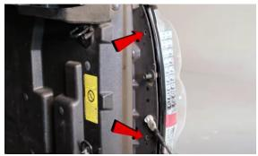
7. Reinstall (2x) phillips screws securing tail light to the body.
