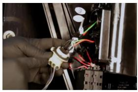
4. Install center bulb insert into center socket making sure to match black wire side of insert to black wire side on socket.
