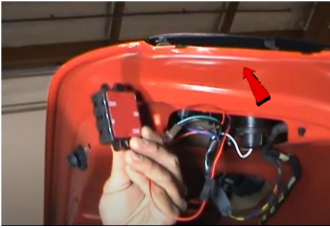
17. Mount resistor using providing 3M tape.
