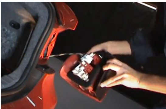
3. Unseat outer tail light and disconnect wiring harness.
