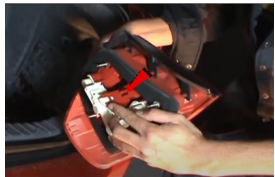
4. Unclip bulb socket plate.
