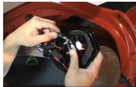
14. Transfer bulbs to Spyder inner tail light.
