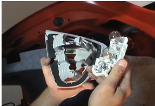
13. Unclip socket plate and remove (1x) small bulb and (1x) large bulb.
