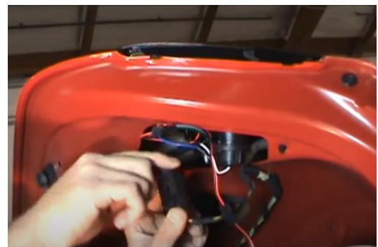
16. Reinstall (1x) 8mm nut and plug in harness.
