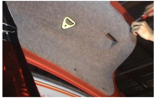
18. Reinstall (8x) retaining clips to secure trunk lid liner.
