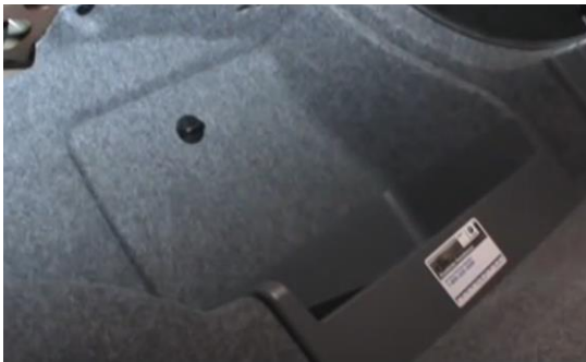
1. Remove thumb screw and access panel.
