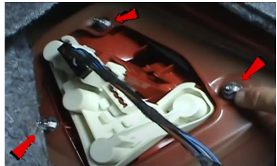
2. Remove (3x) 8mm bolts securing tail light.
