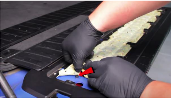
11. Pull back slightly on foam to remove hidden (1x) 8mm bolt.
