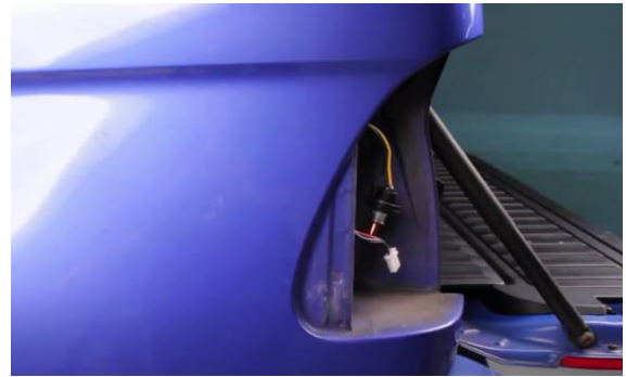
6. Disconnect Red/Grn harness clip and remove turn signal socket from Spyder tail light, thread harness thru body.
