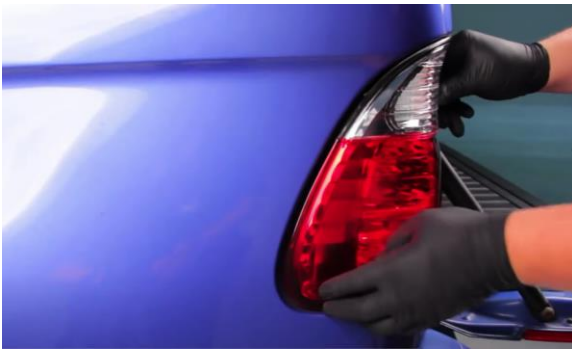
7. Reinstall Red/Grn clip and turn signal socket. Seat tail light making sure not to pinch wires.
