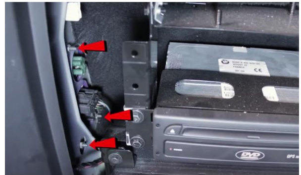
2. Remove (3x) 8mm bolts securing tail light.
